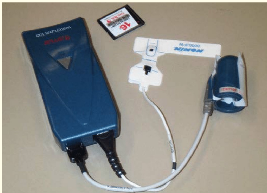
Figure 3: "Watch PAT" Device which acts as Actigram, Oximeter and the peripheral artery tonometer [17].
